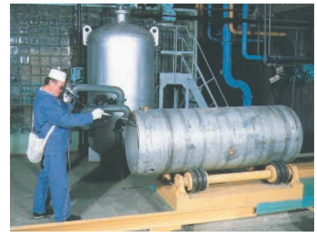
The interior of an LEU-hexafluoride gas shipping container at UEIP is inspected for flaws.
