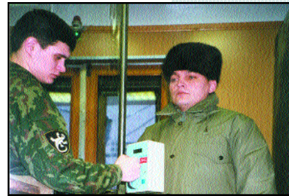
A guard scans a site employee with a hand-held special nuclear material detector.
