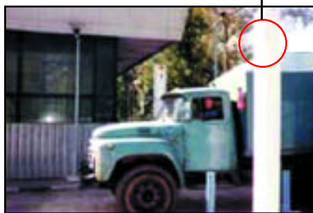
Vehicle portal monitors are used at site entrances to detect special nuclear materials.
