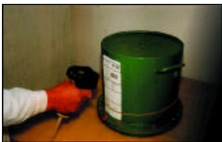
Electronic barcode readers are used to track nuclear material items.
