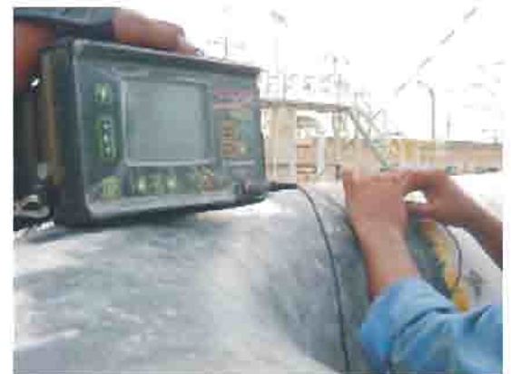
Ultrasonic testing of fuel gas pipe weld at Uch Power Station.
