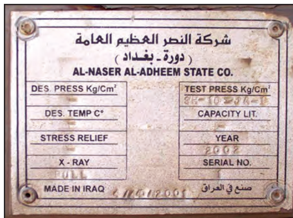
Figure 3 (b). Trailer 1 data plate on reactor vessel.
