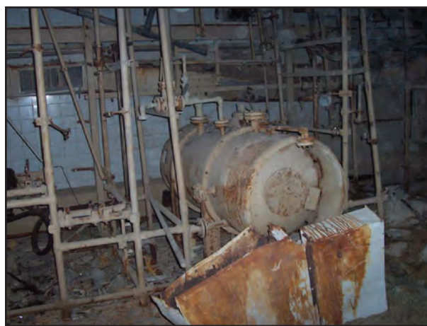
Figure 15. Reactor made from recycled two-ton bulk mustard storage cylinder.
