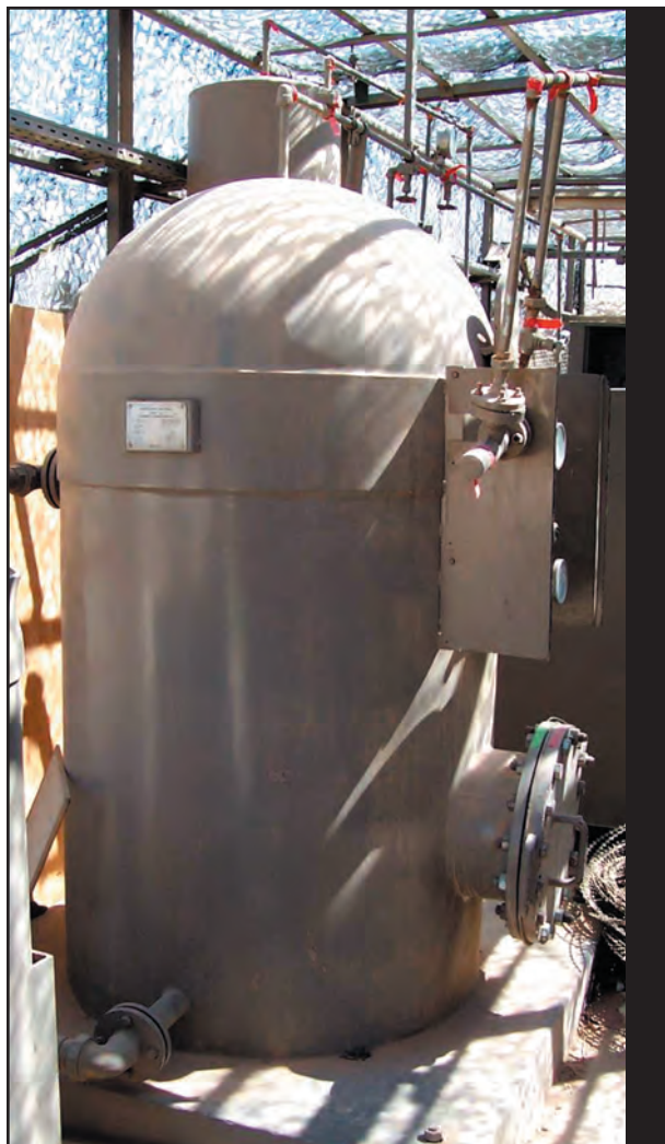
Figure 3 (a). Trailer 1 reactor vessel.
