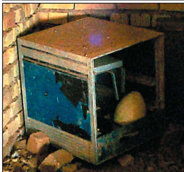
Figure 21. A Skinner Box, a device used to test small rodents who are under the effects of drugs or chemicals, was recovered at one of the sites.
