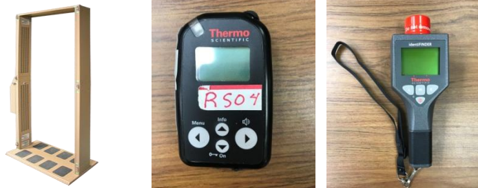
Figure 2. (Left) Portal monitor which can be used to used for Beta/Gamma personnel contamination monitoring and meets the FEMA standard for Emergency Response Portal Monitoring. (Middle) Personal radiation detector that we distributed to our security personnel to detect abnormal radiation level. (Right) Identifinder is used to identify unknown radioisotopes.
